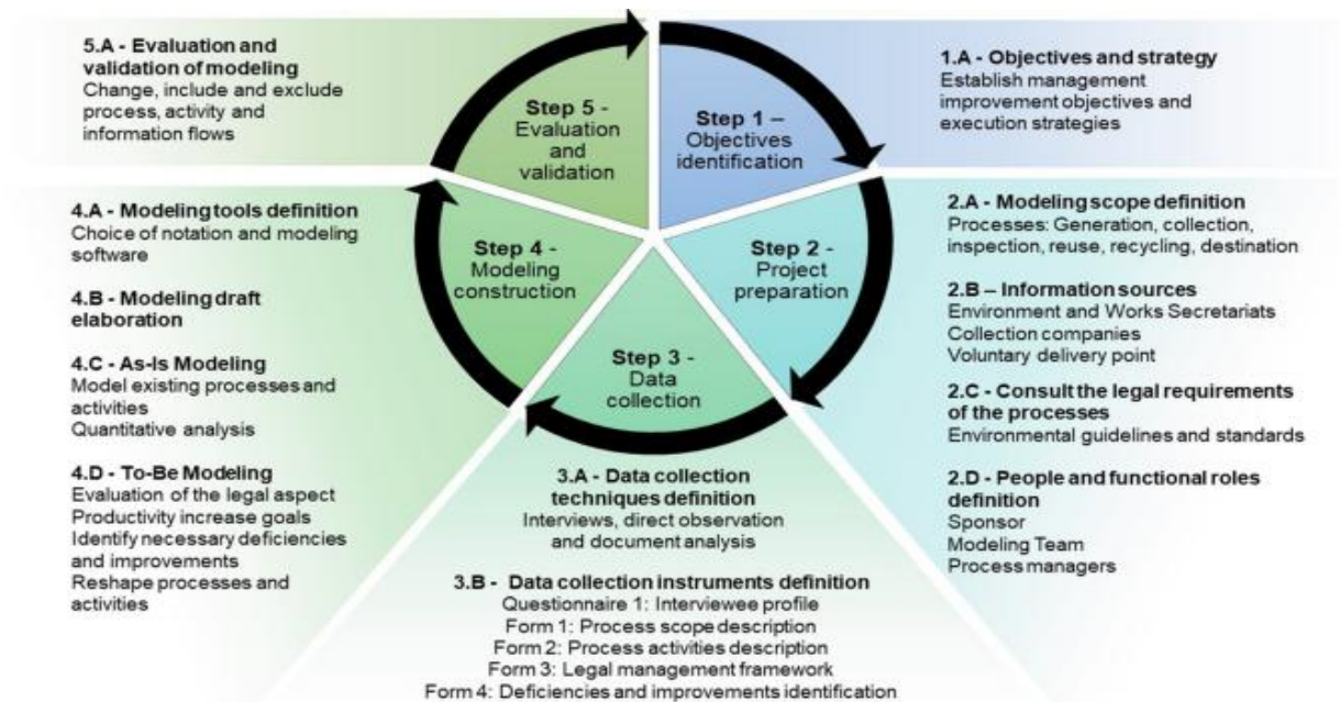
Figure 1 Management of Construction and Demolition waste Materials
